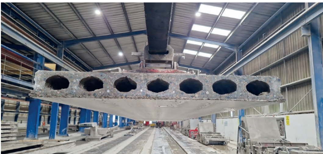
7-holes hollow core slab produced by Nordimpianti's EVO2 Extruders
